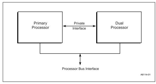
The dual processor pair appears to the system bus as a single, unified processor. The operation is identical to a uni-processor embedded Pentium processor, except as noted in "Summary of Dual Processing Bus Cycles" on page 19-363. The interface shields the system designer from the cache consistency and arbitration mechanisms that are necessary for dual processor operation.
